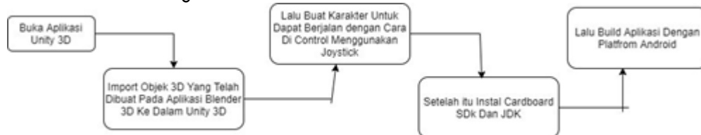
Figure 2. Block Diagram of Application Development in Unity
