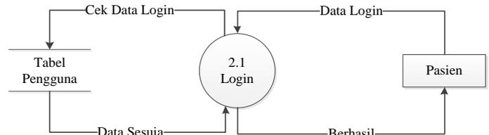
Gambar 5. Data Flow Diagram Level 1 Proses Login
