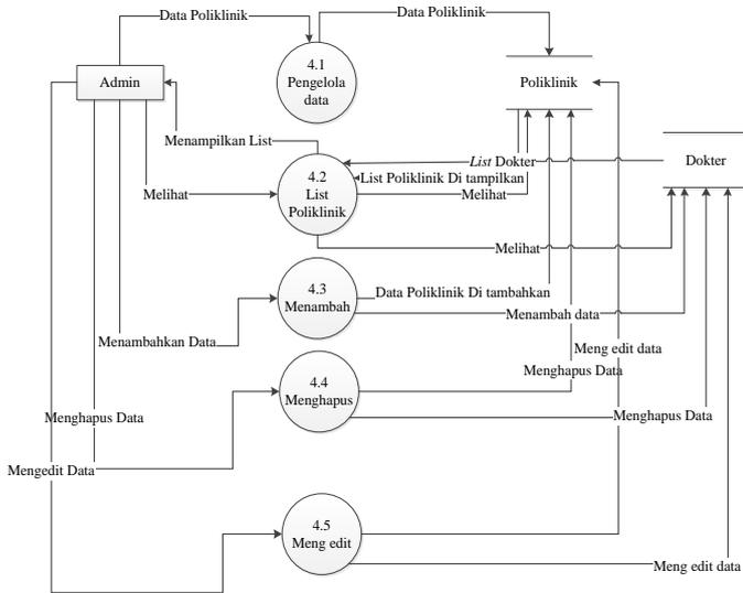
Gambar 7. Data Flow Diagram Level 1 Proses Pengelola Data
