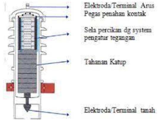
Gbr.2 Bagian-bagian Arrester
