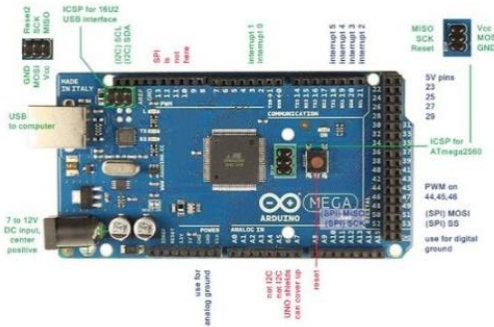
Gbr 2. Board Arduino Mega 2560
