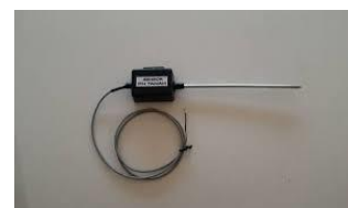
Gbr. 1 Sensor pH Tanah
