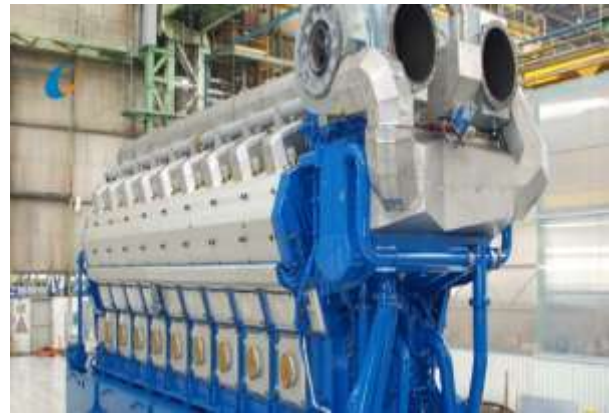
Gbr 3. Mesin Gas Wartsila 50SG
