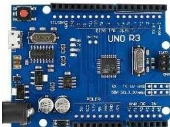
Gambar 1. Board Arduino UNO R3
