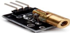
Gambar 1. Sensor Laser
