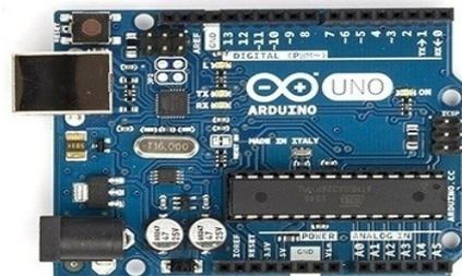
Gambar 7. Board Arduino Uno
