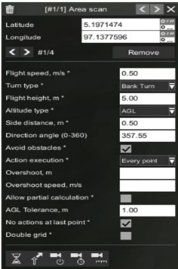
Gambar 17. Detail Area Mapping.
