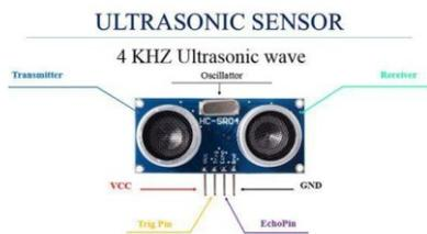
Gambar 6. Ultrasonic Sensor
