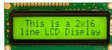
Gambar 4. LCD (*Liquid Crystal Display*) 16x2
