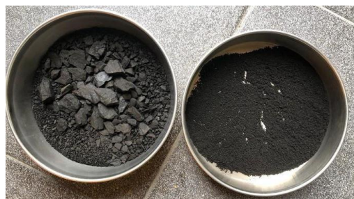
Figure 3. Coal refined to 20 mesh
