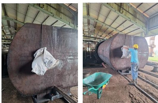
Figure 2. Tbs are hung on trucks for the heating process
