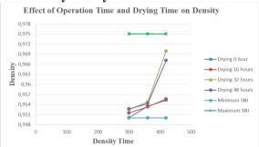
From the picture above, it can be concluded that the density of patchouli oil is in the range of values in accordance with SNI standards and this density has a significant impact on operating time and drying time. The highest density of patchouli oil was achieved in a drying time of 32 hours with an operating time of 420 minutes. Meanwhile, the lowest density occurred when the drying time was 0 hours with an operating time of 300 minutes.
