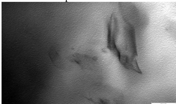
Figure 3.28. TEM photograph of PU/Clay nanocomposites ODA 1 wt%
