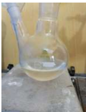
Figure 9. Mixture of water + oil that enters the distillation flask
