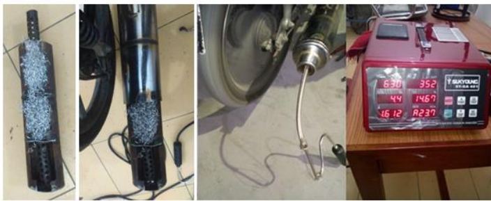
Fig 4. Testing tailpipe using gas analyzer
