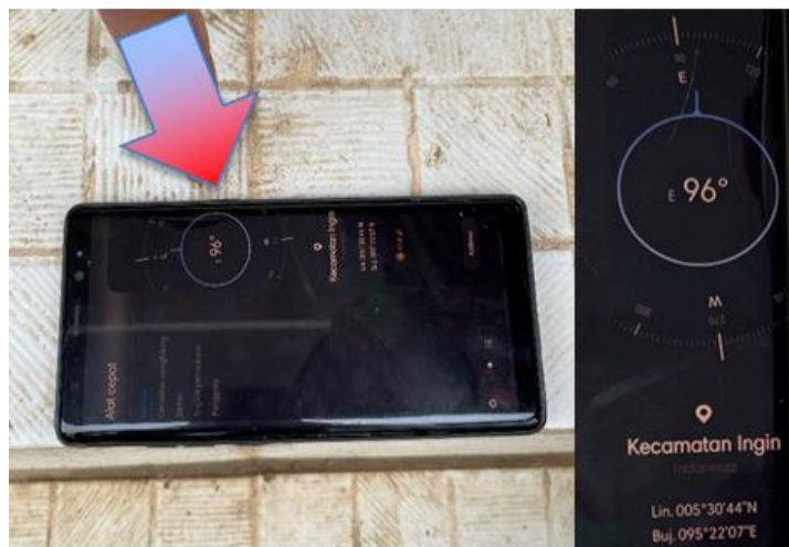
Fig. 5. The azimuth position of the roof solar panels of Dayah Ulee Titi
