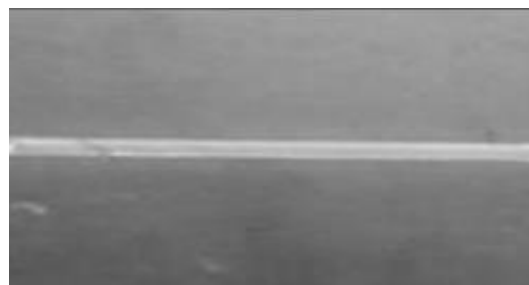
Fig. 3. Welding Results of AA 5083
