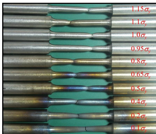
Fig. 10. CD304SS failure type under transient temperature total deformation condition
