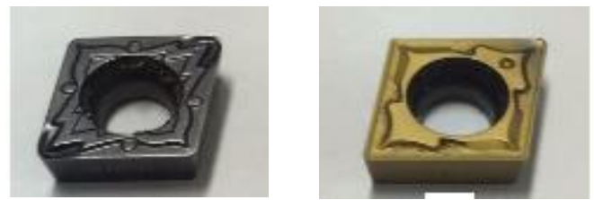
Fig. 3. Insert carbide TiN(a) and TiAlN/Al 2 O 3 (b)
