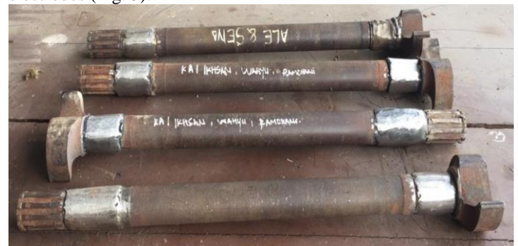
Fig. 5. Material cam shaft which has been hard faced using RB-26 electrodes
