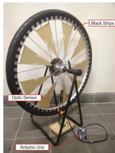
Fig. 5. Paddlewheel mechanics, optical sensors, and Arduino UNO
