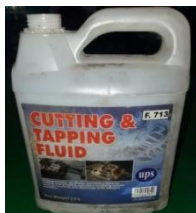
Gambar 8. Cairan pendingin/coolant UPS F.713(cutting & tapping fluid)[10]
