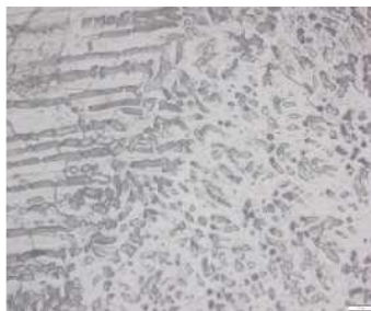
Fig. 1. Formation of chromium carbide on fusion lines and HAZ. [4]
