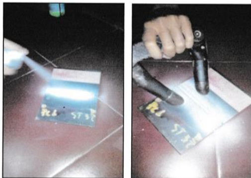
Fig. 5. Inspection of weld defects by Dye Penetrant Testing method, Material ST 37 water cooling medium
