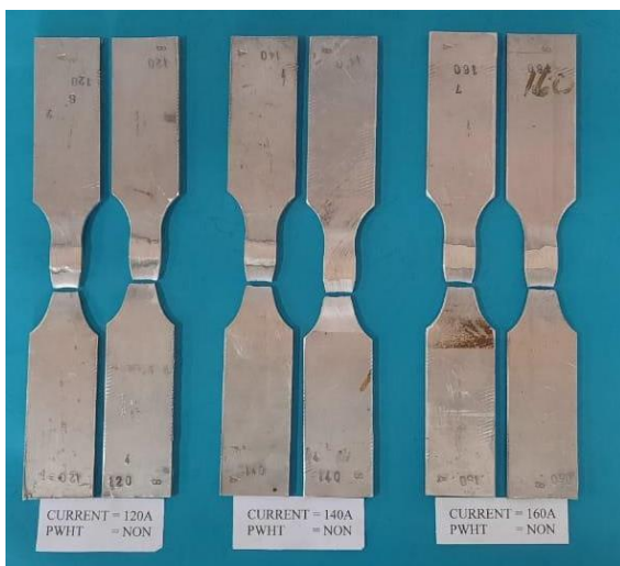
Figure 7. Tensile Test specimen drawing spesimen
